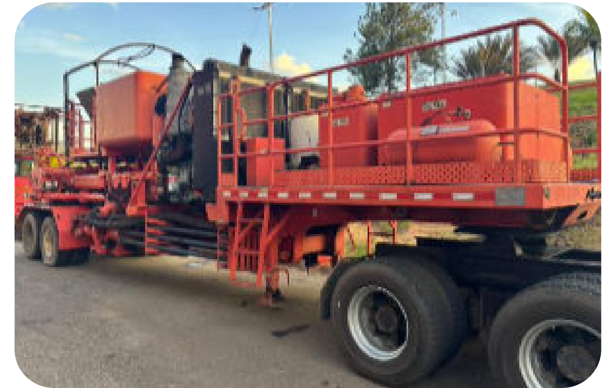
BOMBA DE ALTA PDV-TC-BA-03
