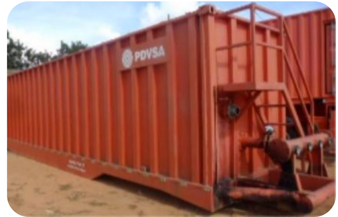
FRAC TANK PDV-TC-FT-07-2
